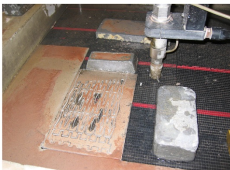
FIGURE 5 . Water Jet cutter with garnet powder
